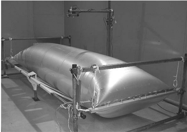
Fig. 14 Test setup of pressurized cylinder test.
